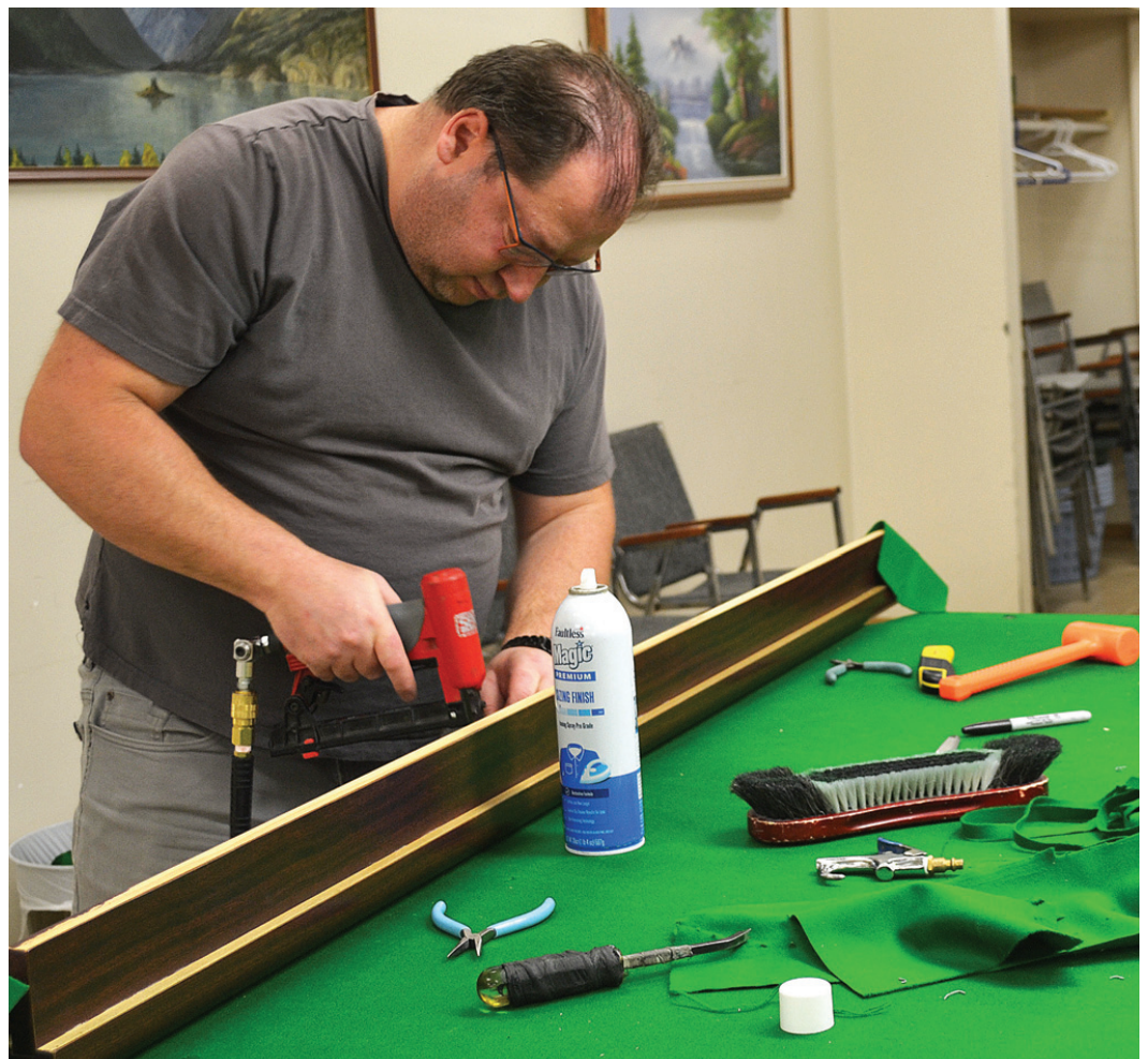
Snooker table repairman Mike Wasoyliw cleans and levels off the shale which makes the 2,000 lb. table so heavy. PATRICIA HARCOURT PHOTOS
